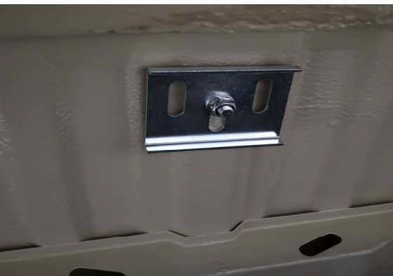
Reinforcements mounted in the middle position (Under the spare wheel)
