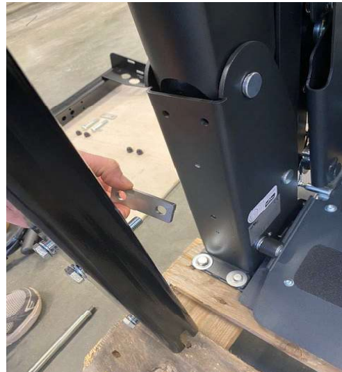
Place spacer between bracket and lift.
