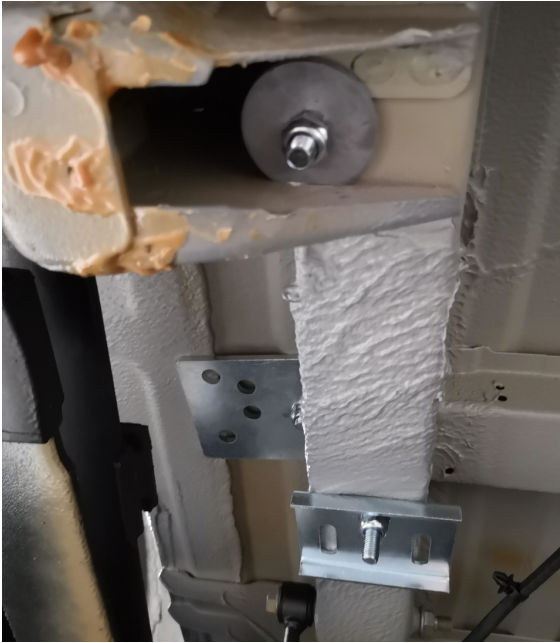
Reinforcements mounted on the left side. (Reinforcement plates are not included)
