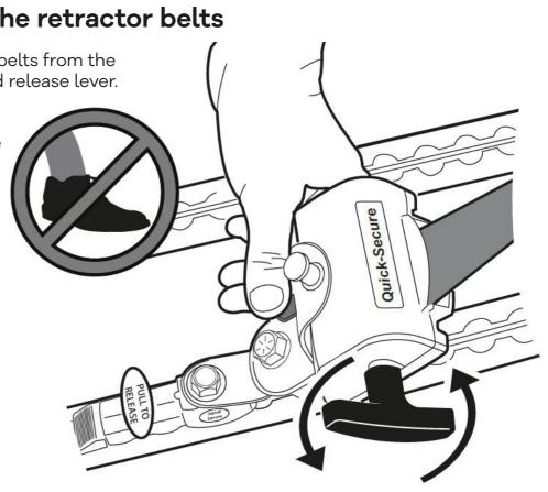
NB! Press the lever only by hand – do not step on it.
