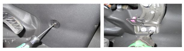
Handi brake is mounted on the extended screw.
