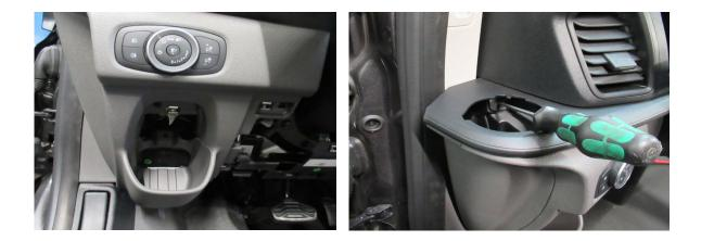
Drill Ø 21mm hole for operating switch "Handi Brake" as shown in picture
