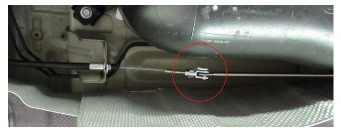
Drawbar is adjusted at original assembly point. Be aware that the Handi brake is fully released.
