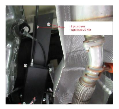
Scrap the original hand-brake wire.
