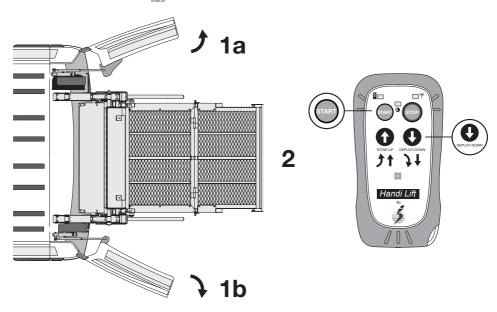
2. Continue pressing the button . When a small safety-delay occurs, keep pressing to close the doors completely.
