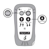
2. Continue pressing the button until the vehicle doors are fully open and the wheelchair lift is completely unfolded.
