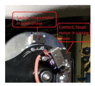
Stop switch (Open) is adjusted so that the motor stops running about 10-20 degrees before the top.
