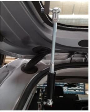
Fit pull arm from HDO. Note position in closed condition. Stop switch (Close) on HDO is adjusted so motor stops pulling about 30 - 40 degrees before fully closed. (Then the gas damper close the tailgate / Hatch.)
