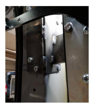
Mount the HDO bracket on the left rear pillar (D Pillar)
