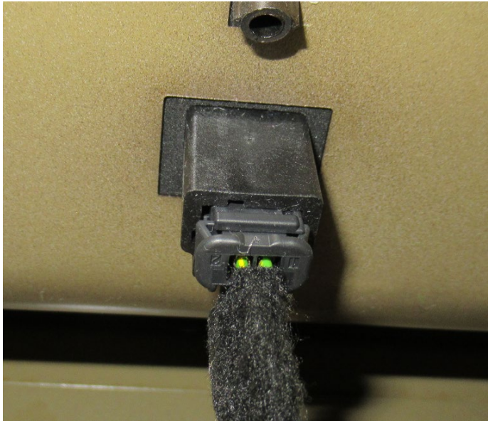
Door handle. Ground signal "input" pin 1 (Door release)
