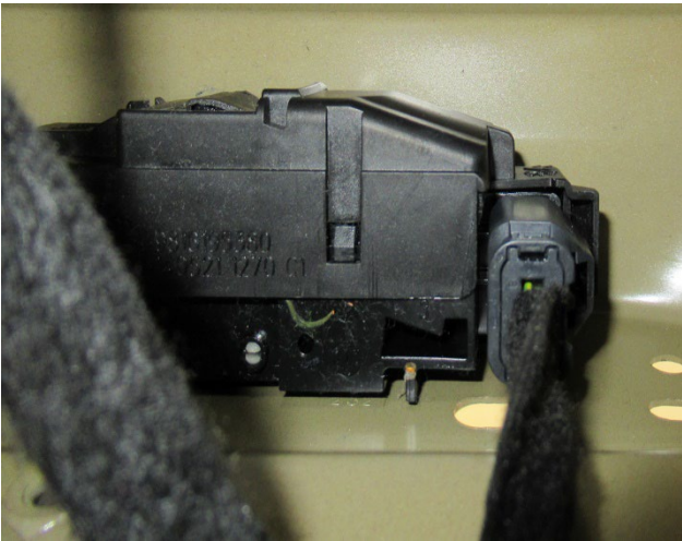
Door lock. Return signal pin 3 = Ground signal/door is open.
