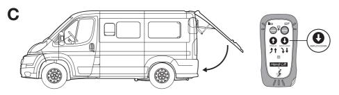
C. Press and hold the button • to close the hatch door.
