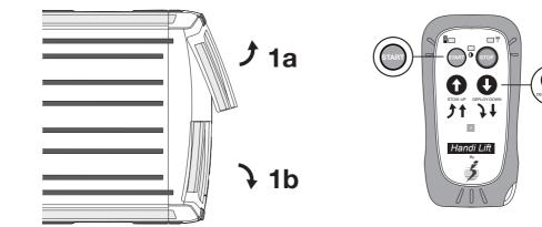
2. Continue pressing the button out in the vehicle doors are fully open and the wheelchair lift is completely unfolded.
