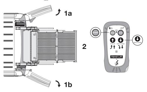
2. Continue pressing the button  $\bigoplus_{\text{score}}$ . When a small safety-delay occurs, keep pressing to close the doors completely.
