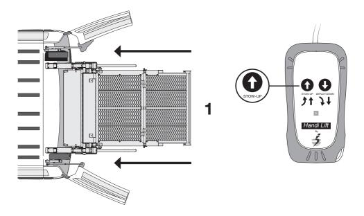
2. Continue pressing the button . When a small safety-delay occurs, keep pressing to close the doors completely.
